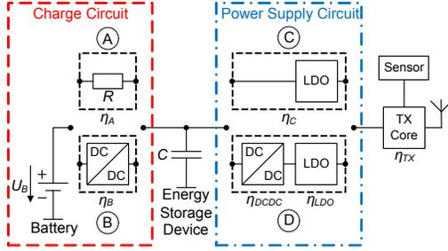
Fig. 1. Supply Concepts for a Transmitter node:
