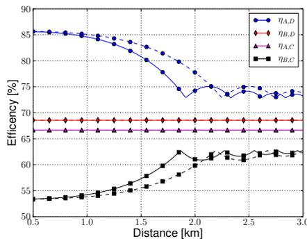
Fig. 2. Efficiencies of the different power concepts with  $\eta_B = 0.8$ ,  $\eta_{DCDC} = 0.9$ , number of bits  $k = 100$ ,  $F = 10$ ,  $(E_b/N_0)_{RX} = 1.5$ ,  $\eta_{TX} = 0.15$ ,  $U_U = 3.0$  V,  $U_L = 2.1$  V,  $U_{LDO} = 2.0$  V and  $L$  along Okumura-Hata model. The size of the capacitor  $C$  is  $680 \mu\text{F}$  for the continuous lines and  $1200 \mu\text{F}$  for the dash lines.
