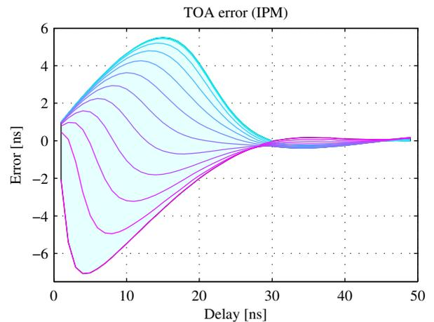
Fig. 2. TOA estimation error for the IPM. The TOA error is shown for delays up to 50 ns and phases from 0 to 165° in steps of 15° between the 2 propagation paths. Both paths are equal in amplitude.
