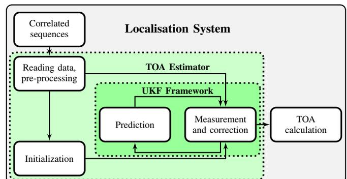
Fig. 1. Integration of the TOA estimator into the localization system.
