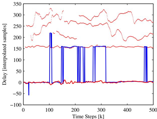
Fig. 5. Comparison of tracking performance of the UKF (red) and inflection point algorithm (blue). Dark lines show the LOS estimate. Up to three delayed propagation paths are tracked in addition to the LOS path by the UKF.
