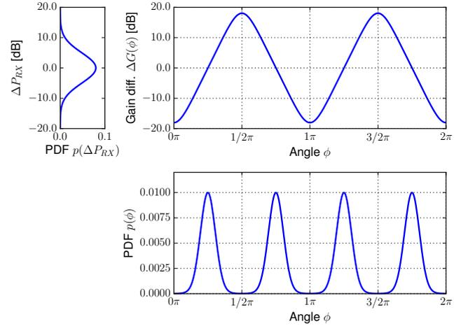
Figure 3: PDF for direction estimation: Exemplary measurement error distribution, gain difference function  $\Delta G(\phi)$  and the DOA PDF  $p(\phi)$  at  $\sigma = 5$  dB and an observed RSSI difference of  $\Delta P_{RX} = 0$  dB.
