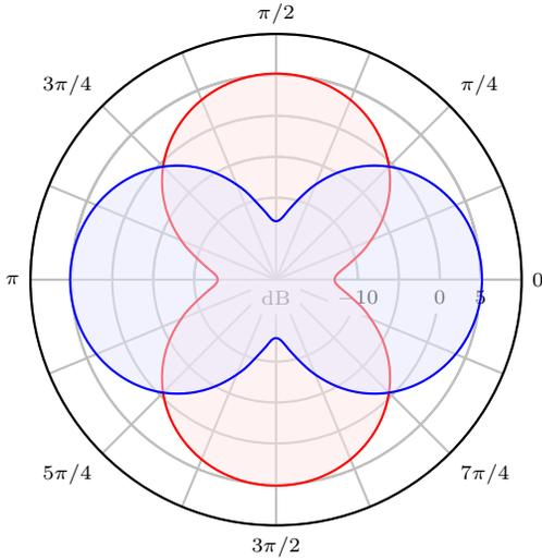
Figure 2: Far-field antenna gain patterns  $G_{RX,1}(\varphi)$  (blue) and  $G_{RX,2}(\varphi)$  (red) for a antennas provided by a dipole array with a radius of  $r = 0.23\lambda$  and at a rotation angle of  $\nu = \frac{1}{2}$  between the two antennas.
