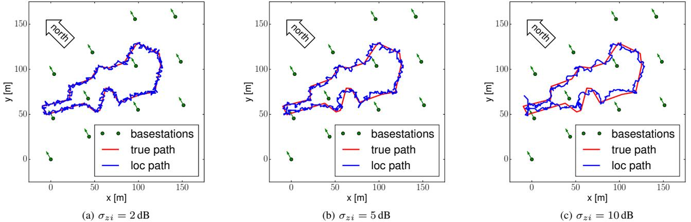
Figure 7: Reference trajectory (red line), the estimated trajectory of grid-based filter (blue line) and sensors nodes (green dots). Fading levels of  $\sigma_{z_b} = 10$  dB and  $\sigma_{z_i} = \{2 \text{ dB}, 5 \text{ dB}, 10 \text{ dB}\}$
