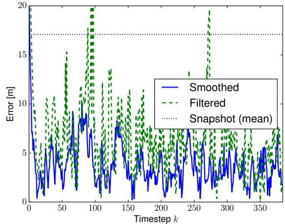
Figure 8: localization errors by way points for a forward filter implementation and a forward-backward smoothing filter implementation
