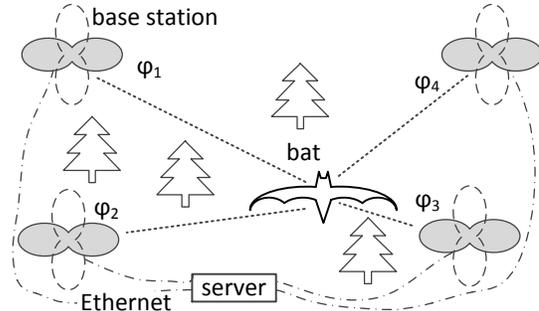
Figure 1: Bats localization system with four base stations connected by Ethernet to a central server
