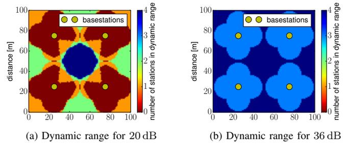
Figure 3: Coverage map for  $100 \times 100$  m with four base stations
