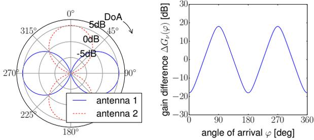
Figure 2: Antenna pattern and gain difference function
