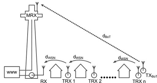
Fig. 1. BoT principal and WSN principal with  $n$  nodes and the different propagation conditions. For the BoT principal a receiver on a exposed poison like a television tower is shown.
