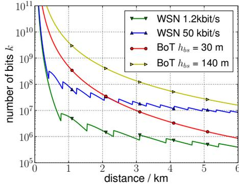
Fig. 2. simulation results: possible transmitted bits  $k$  with the energy of a single coin cell for BoT and a multihop WSN
