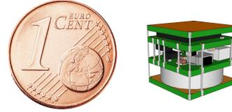
Fig. 3. Hardware demonstrator  $1 \text{ cm}^3$  cube with coin cell, power supply circuit, micro-controller, RF-Chip and antenna compared to a 1 cent coin [www.ecb.int]
